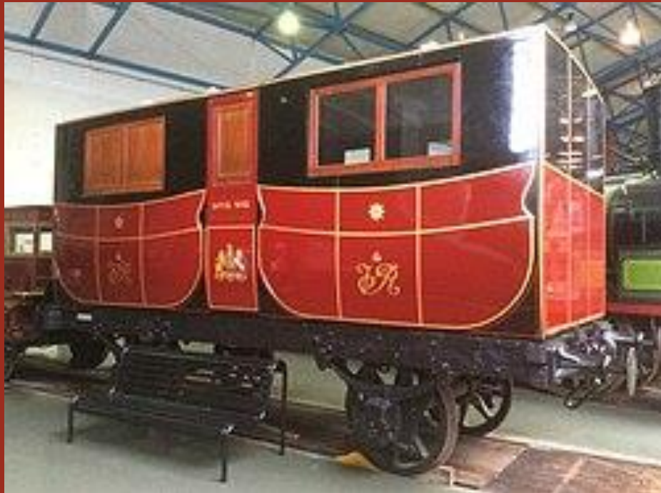
Replica of 1838 Grand Junction Railway travelling post office van
